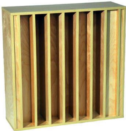
Fig. 18. RPG Modfuser. This is a typical diffuser that spreads sound horizontally. If it's turned 90 degrees it will spread sound vertically instead. The dimensions of the cavities are mathematically determined. Photo: www.rpg-europe.com
