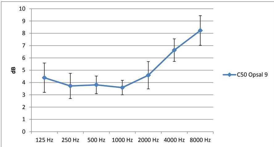
Figure 2: Clarity in operating room 9. Average values and standard deviations are shown for C50.
