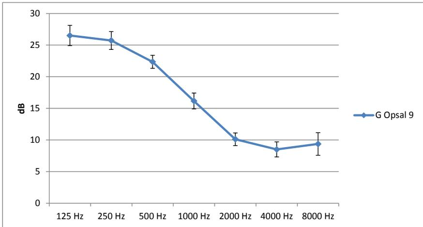
Figure 3: Sound strength in operating room 9. Average values and standard deviations are shown for G.
