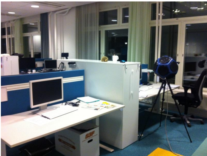
Figure 5 Measurement path 4.2 – loudspeaker placement
