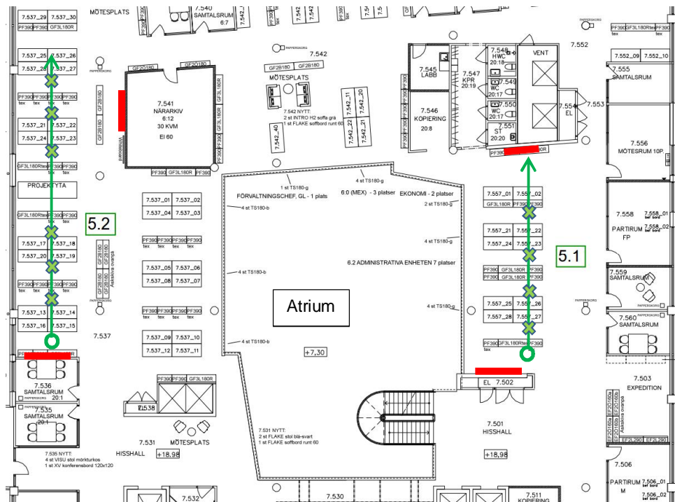
Figure 2 Location of measurement paths and on floor 5. Sound absorbing wall segments are marked with red.
